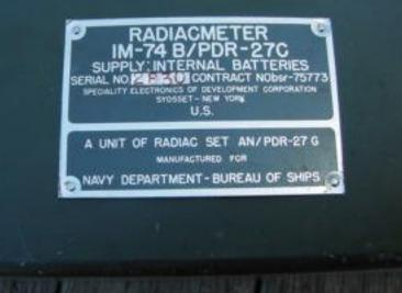
The AN-PDR27 meter has been a standard US military issue radiation survey meter or Radiac for the past 45 years. *Radiac is an acronym for* "*Radiation, Detection, Identification, And Computation*".
