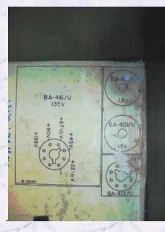
The battery well of the meter looks like the picture below when all the batteries I cobbled together are in it. If you want a small discussion on powering up surplus military equipment that utilizes weird batteries, <u>go here</u>. It's nice to know how to make things "go" if you don't have quite the right parts.
