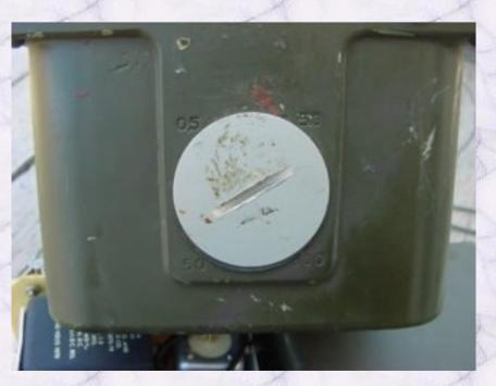
This meter has no high voltage adjustment capability to adjust the voltage to the GM tubes. The usual method was to replace the tubes when they aged enough to not calibrate when sent back to the depot. But due to the long life of the 5979 tubes this was usually not a problem over the life of the meter.
