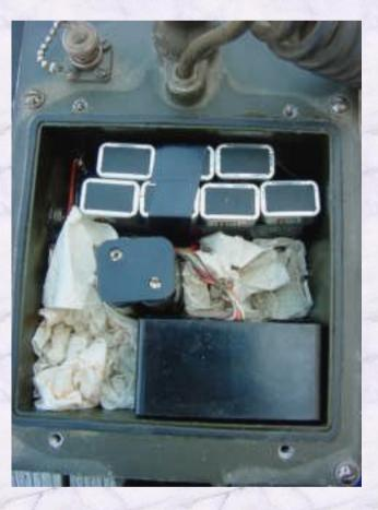
In of the picture below the135 volt battery is in the top with the 22.5 volt battery below it.
