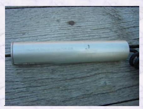
The probe is setup such that there is a shutter assembly at the end and to detect the presence of Beta radiation the "beta window" is opened
